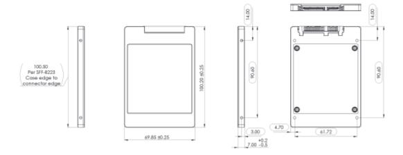
The figure below is enlarged to show detail, but is not the actual size of the form factor. This figure shows 2.5"/7mm cased one-half form factor (for 250GB and 512GB capacities only).
